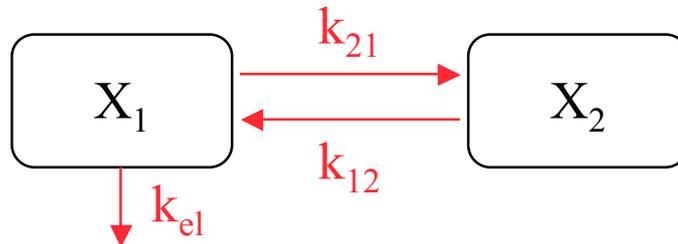
$$\begin{aligned} \frac{dX_1}{dt} &= k_{12} \cdot X_2 - k_{21} \cdot X_1 - k_{el} \cdot X_1 \\ \frac{dX_2}{dt} &= k_{21} \cdot X_1 - k_{12} \cdot X_2 \end{aligned}$$
