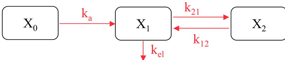
$$\begin{aligned} \frac{dX_0}{dt} &= -k_a \cdot X_0 \\ \frac{dX_1}{dt} &= k_a \cdot X_0 - k_{21} \cdot X_1 - k_{el} \cdot X_1 + k_{12} \cdot X_2 \\ \frac{dX_2}{dt} &= k_{21} \cdot X_1 - k_{12} \cdot X_2 \end{aligned}$$
