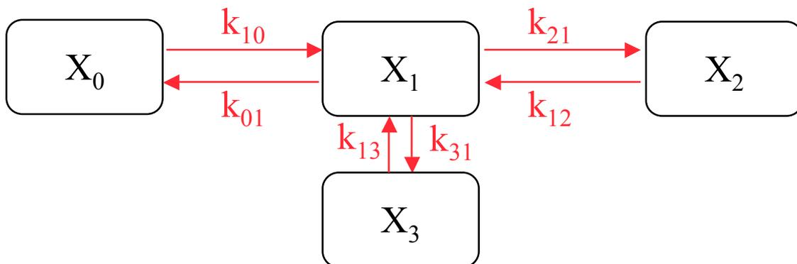
$$\begin{aligned} \frac{dX_1}{dt} &= k_{10} \cdot X_0 - k_{01} \cdot X_1 - k_{21} \cdot X_1 - k_{31} \cdot X_1 + k_{12} \cdot X_2 + k_{13} \cdot X_3 \\ \frac{dX_2}{dt} &= k_{21} \cdot X_1 - k_{12} \cdot X_2 \\ \frac{dX_3}{dt} &= k_{31} \cdot X_1 - k_{13} \cdot X_3 \end{aligned}$$
